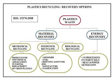
The choice between Mechanical Recycling, Feedstock Recycling or Energy Recovery will depend on the types of plastics waste and the relative ease / difficulty in total or partial segregation of different groups of plastics materials from each other or from other waste materials / contamination.
